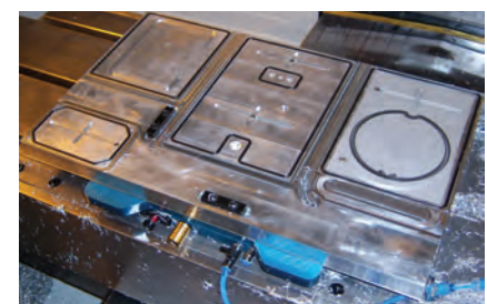
Custom vacuum pallet with 4 vacuum chambers on VM300
