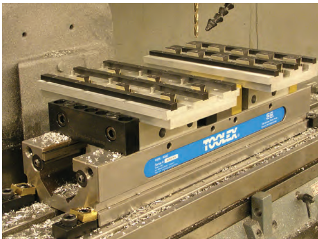
Fixtured with Mitee-Bite Uniforce® Clamps and locating rails
