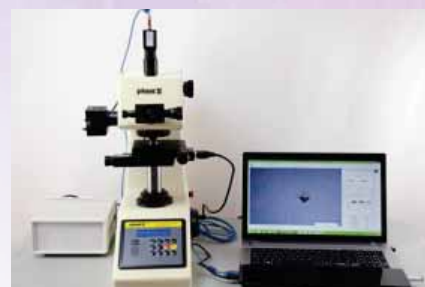
Motorized X-Y Stage w/Controller and Measurement Software Includes Video cam, Adapter and Turret Control w/ Auto-measure software Part No. 900391-ESOFT
