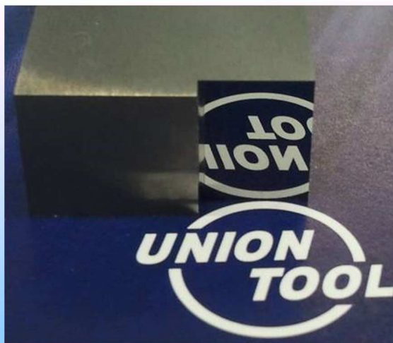
Material: 90HRA (CIS VM-40) Cemented Carbide
